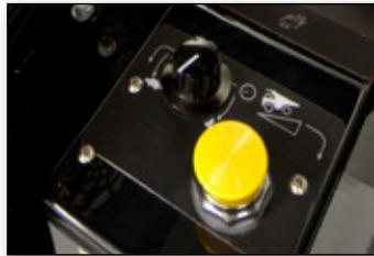
*Gear selector and hoist control levers*
