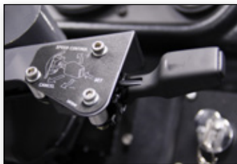
Automatic speed controls
