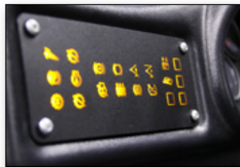
Warning light cluster displays machine health
