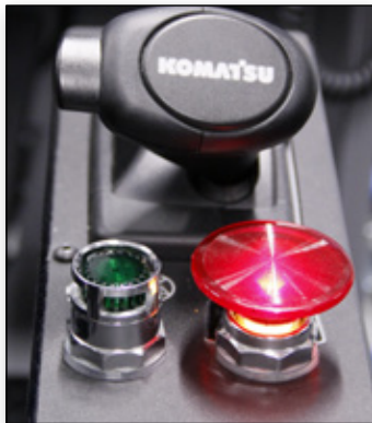
Gear selector and emergency shutdown
