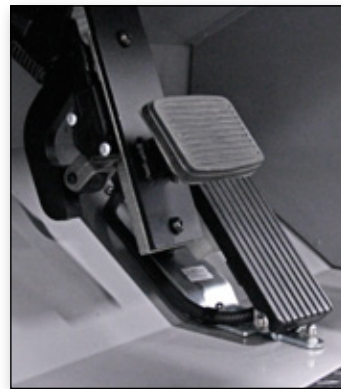
Throttle and retarder/service brake pedals match real machine cab
