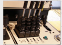
Mast, levelling jacks & throttle levers
