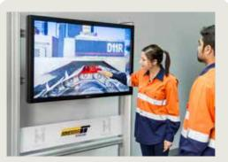
Immersive Technologies developed a touch screen Pre-Start inspection tool after customer feedback indicating worn and damaged components were not being reported and they needed something to train operators to recognize problems before they become costly to repair. This tool and a myriad of others will now be part of Immersive Technologies' new Learning Systems business unit
